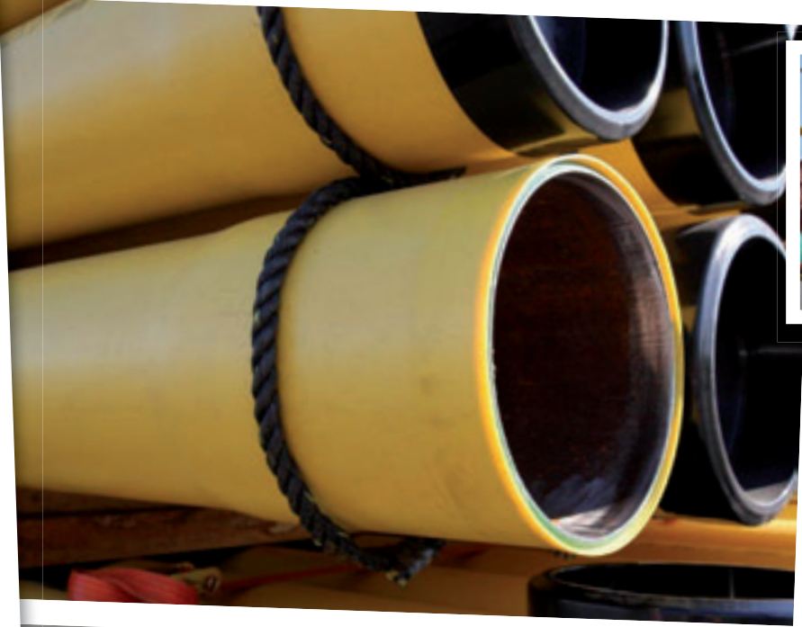
Left: The bell ends of the HDPE-coated Zap-Lok® pipes were provided with an approximately 10 mm plastic coating overlap and corrosion protection of the pipe end bevel. The black plastic caps are designed to protect the pipe ends from damage. Top: Pipe loading at the port of Antwerp
