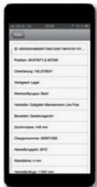
4 Using the logged data, it is possible to compile a pipe list and a complete pipe book. In addition, data from other pipeline internals such as valves, fittings or bends and special features of the pipeline route can also be stored.
