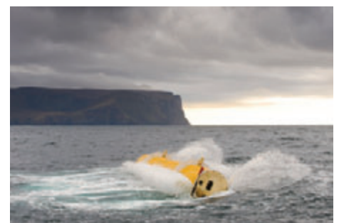
The Oyster wave energy converter pumps seawater to an onshore turbine for the production of electricity.
