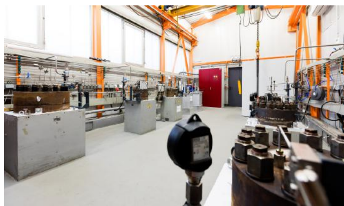
Test setup for CO 2 corrosion tests (rotating cage) and autoclave laboratory at Salzgitter Mannesmann Forschung GmbH
