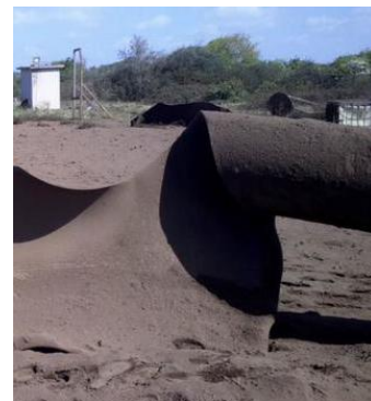
Burst test on a CO 2 test line. CO 2 mixture ( 94.0% CO 2 ) at 127 bar, material X65, measuring 610 x 13.7 mm, from the RFCS-funded SARCO2 project. Cracking in the steel pipe is arrested after a few meters.
