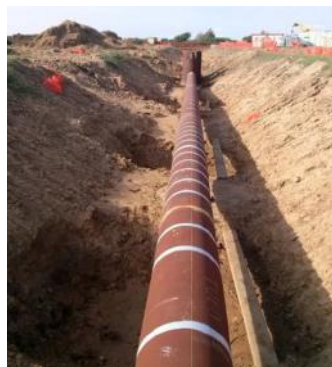
Burst test on a CO 2 test line. CO 2 mixture ( 94.0% CO 2 ) at 127 bar, material X65, measuring 610 x 13.7 mm, from the RFCS-funded SARCO2 project. Cracking in the steel pipe is arrested after a few meters.
